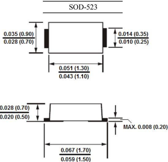
Dimensions in millimeters and (inch)
